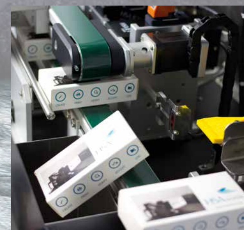
Blow-out Reject. The catch tray guides rejected cartons into the bin.
