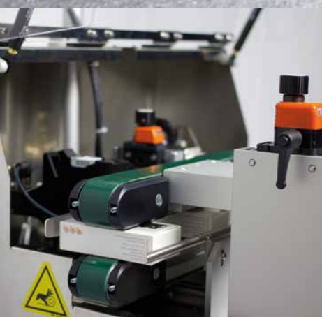
The top belt is height adjustable from 10 to 75 mm. Synchronized carton guide between top and bottom belts.
