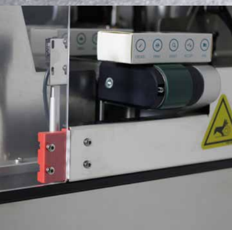
Safety switch will stop the machine if cover is opened during production.
