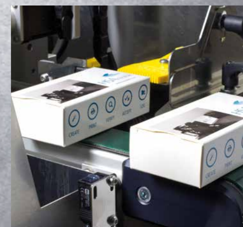
Accept verification sensor.
