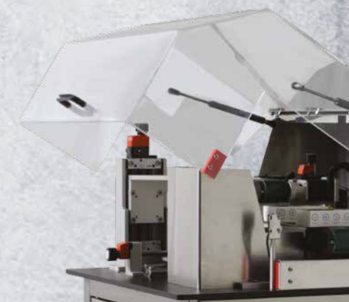
Transparent top cover and safety guard.
