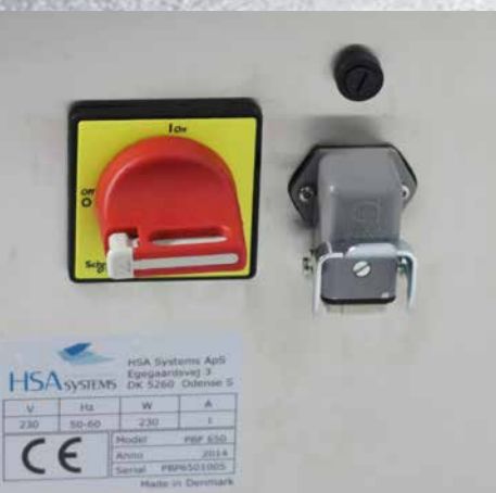
Main power On/Off, Fuse and Main power connections are found on right side of the machine.
