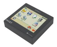
Our Premium MTHP4 MiniTouch controller is robust and well-suited for harsh industrial environments. The MiniTouch controls printheads of up to 50 mm print height and is ideal for being integrated into packaging lines, webs, inserters, folders or collators.
