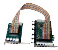
The CB6e board is based on PCI express and can control up to 4" of print height. For additional print height, a plug-board can be connected to increase the print height by an additional 4", providing a total print height of 8" via one controller board.
