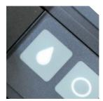
Purge button on each printhead From the printhead keypad, each cartridge can be purged individually.
